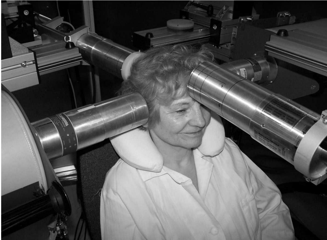
Figure 3: Typical arrangement of 4 HPGe for in vivo measurement of low energy photon emitters such as ^{210}\text{Pb} , ^{241}\text{Am} and isotopes of Pu in the skull [74]
